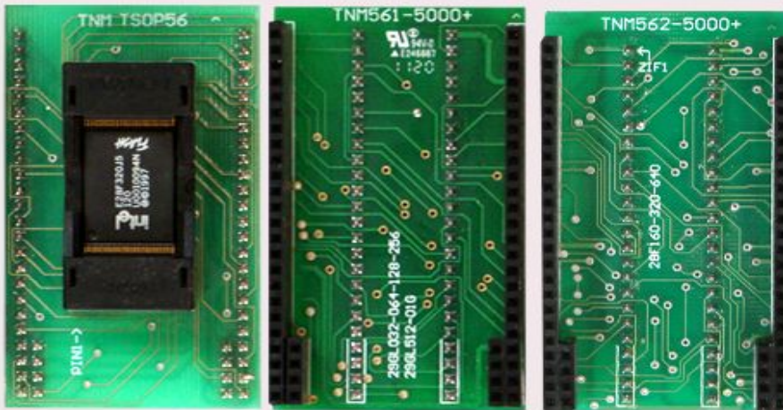
All 56 Pins TSOP Type1 (20mm) Can be programmed by Economic Adaptor Model ADP556T2 with different bottom plates.
